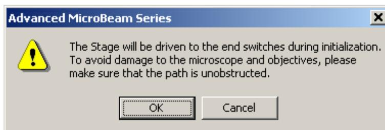
6. Click its OK button. The stage drives to the lower limit switches, then reverses and drives to the upper limit switches, and finally the stage returns to the original coordinates.
