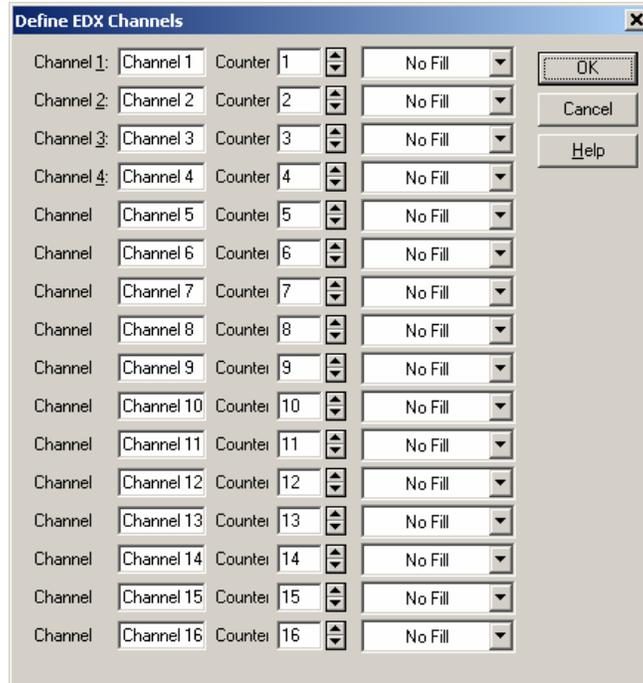
16. Type in the element designation in the Channel box, the Counter number indicates the spectrometer designation and finally click the down arrow by the No Fill box to modify the color displayed for each x-ray.
