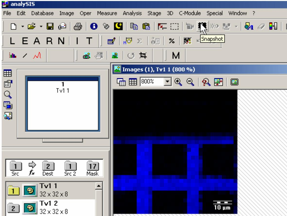
31. Next the operator will define the area to scan. In this example we will collect a 1mm x 1mm grid. Move the stage to the center point of the area of interest.
