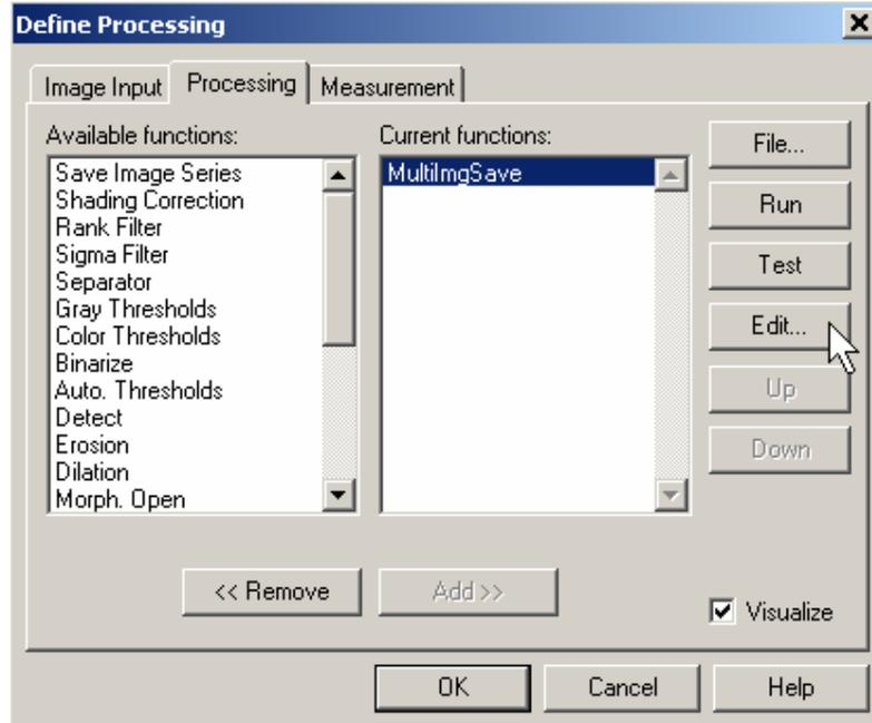
**43. The MultiImgSave function should appear under current functions list. Click the MultiImgSave function and then click the Edit... button. This opens the MIS Folder dialog. Here the destination folder for your images is created or selected.**
