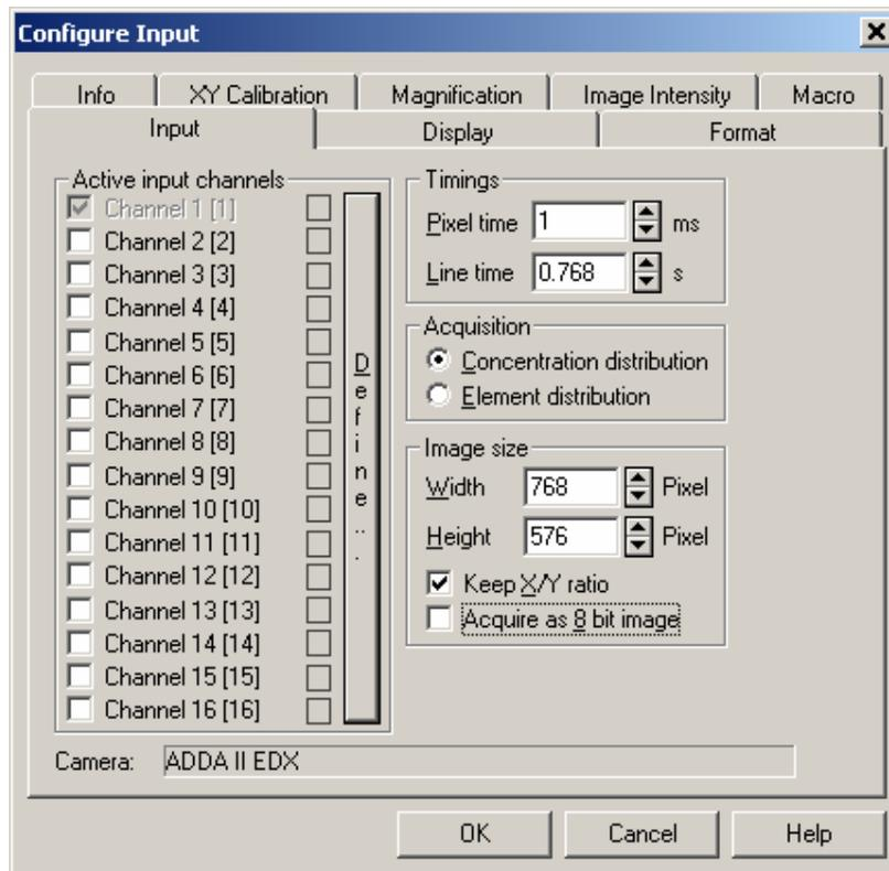
15. Check the correct number of Active Input channels (spectrometers for mapping) and click the Define bar to edit the label and color schemes in the Define EDX Channels window.
