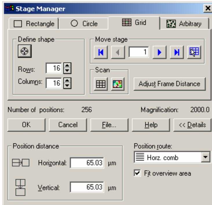
34. With the stage set in the center of the 1mm x 1mm area, click the Set Center button in the Define shape portion of the window.
