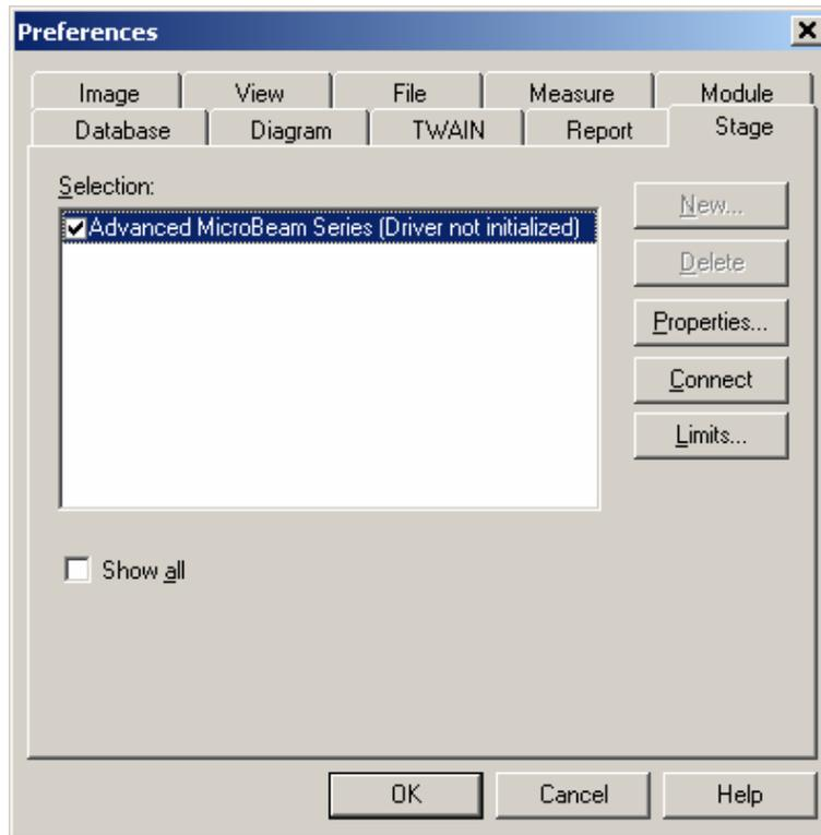
4. The stage driver requires initialization. Click the Limits button. The Advanced MicroBeam Series driver window appears.
