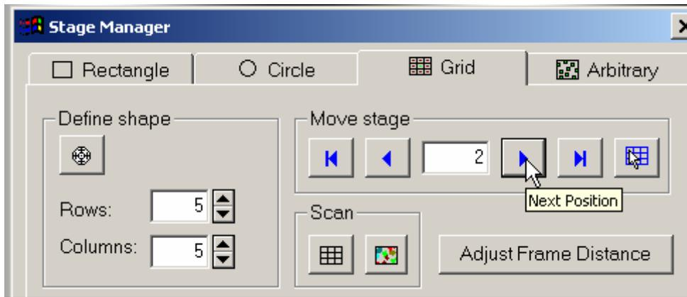
**4. Click the Next Position button to move the stage to the center of cell 2.**
